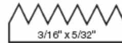
3/16" x 5/32" V Notch 3 ply and 5 ply Engineered Plank Coverage: 50 sq. ft. per Gallon
